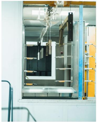
• Cycle Time: 8 FPM - 1550ft of conveyor - 1 automatic spray booth - 2 manual spray booths
